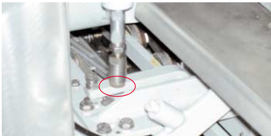
"Puffer" af metal, der rammer polyethylenklods.
